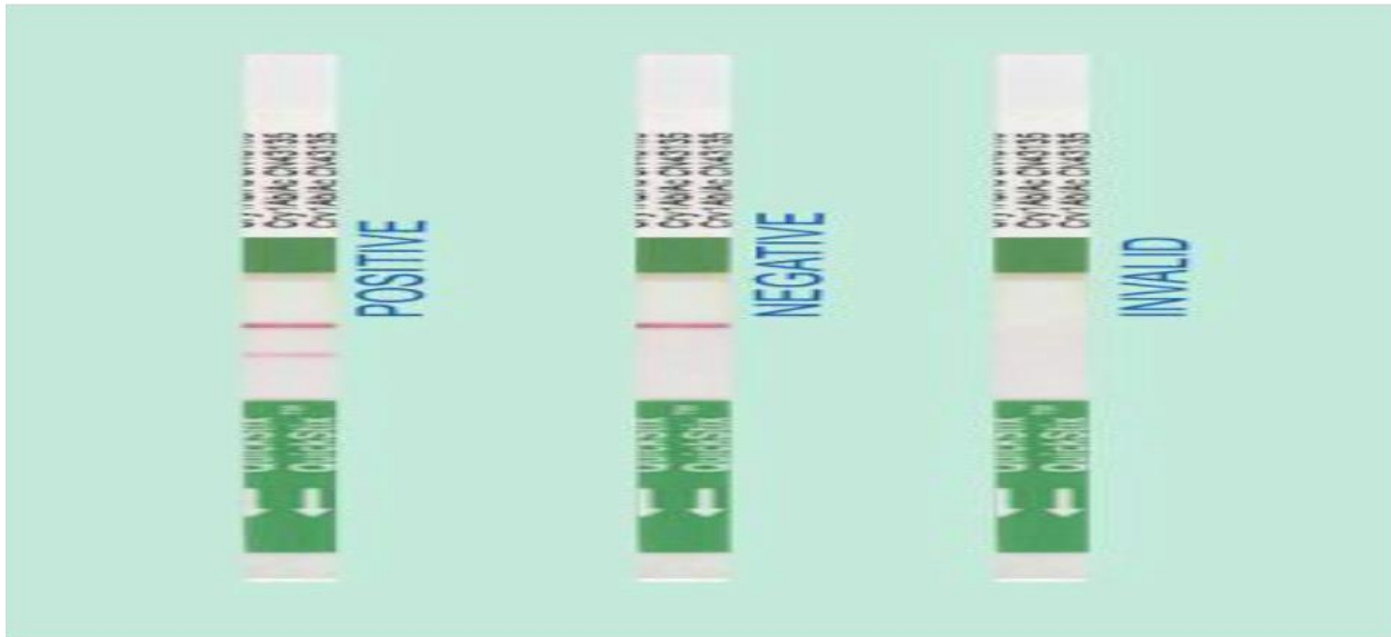
Figure 1. Cry1Ab/1Ac Bt strips showing positive, negative and invalid result (Enviroligix, 2008).
