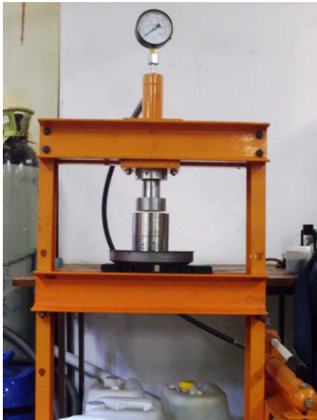
Figure 1. Custom-built hydraulic cold press.
